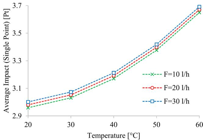
**Fig. 4.** Environmental impact of lab-scale plant in function of temperature and water flowrate.
