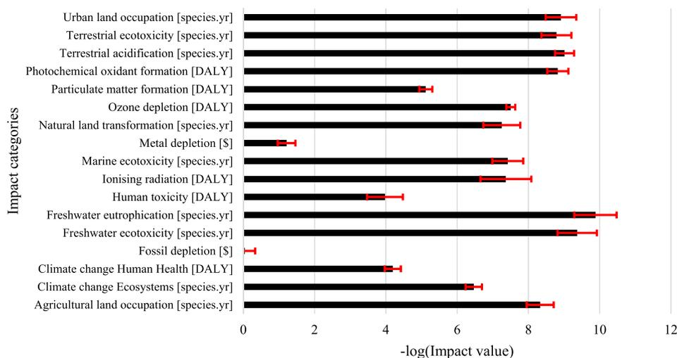
**Fig. 6.** Midpoint impact results of the LCA analysis performed with the parameters of scenario 26 (water flowrate = 30 Lh<sup>-1</sup>, T = 20 °C and P = 450 mmHg). The X axis is a negative logarithm, i.e. the higher the value, the lower the impact.
