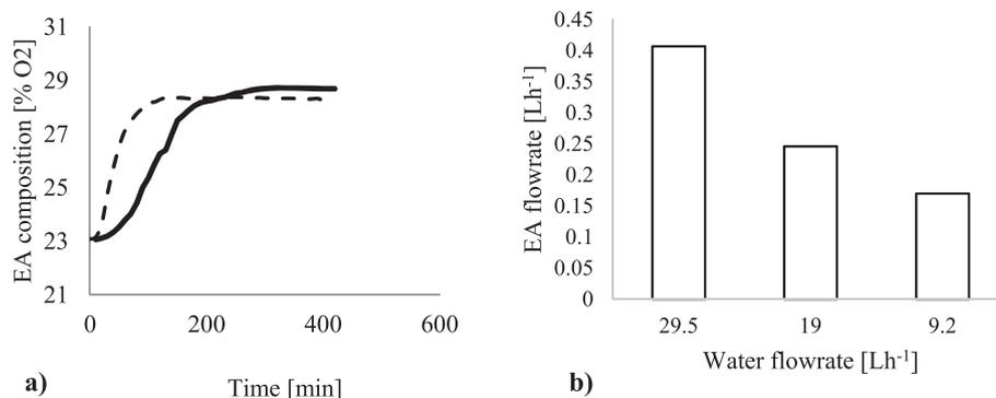
**Fig. 3.** Experimental results: a) EA oxygen composition at different pressures, 500 mmHg (dotted line) and 300 mmHg (full line) and b) EA flowrate at different inlet flowrates (data obtained at  $T = 50^\circ\text{C}$  and  $P = 300 \text{ mmHg}$ ).
