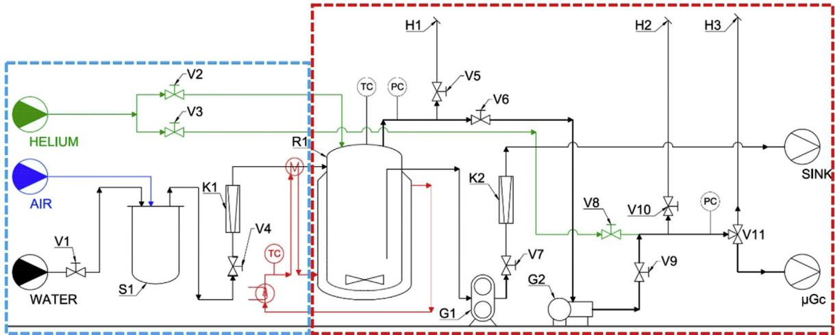
**Fig. 1.** Flowsheet of the experimental setup, V1-11: valves, S1: equilibrating vessel, R1: degasser, K1-2: liquid rotameters, G1: liquid pump, G2: vacuum pump, H1-3: purge. Blue dotted line indicates the water enrichment section while red dotted line the EA desorption one. (For interpretation of the references to colour in this figure legend, the reader is referred to the web version of this article.)
